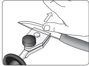
Hold the knife and the jig as illustrated. Make sure that you press your thumb (or palm) on the jig so that it is always pressed against the back of the Universal Support. Move the knife slowly back and forth over the grinding wheel. Ensure that the blade is in contact with the entire width of the wheel. Raise the knife handle when grinding the tip of the knife.
