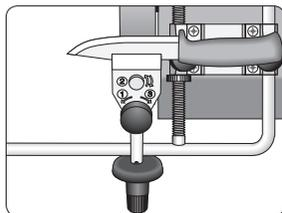
Move the Universal Support to the honing wheel side. Set the jig so you get the same honing angle as grinding angle.
