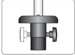
Earlier design with locking screw. (The new design is self-locking.)
