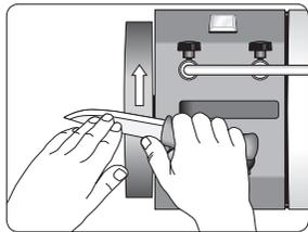
Turn the machine around. Dismount the knife. Hone and polish the bevels on the leather honing wheel. Let the entire bevel touch the leather wheel, so you hone at the same angle as at the grinding. Move the knife back and forth a few times on each side of the blade until the burr disappears.
