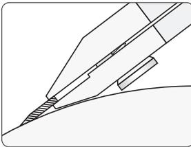
The jig needs to grip the knife with min 2 mm ( $\frac{5}{64}$ " ). You can grind knives with a width down to 14 mm ( $\frac{9}{16}$ " ) with an edge angle of 25°. Knives with narrower blades, see SVM-00 page 59.
