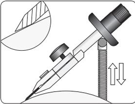
Set the Universal Support so that the heel of the bevel touches the grinding wheel.
