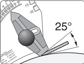
Set the desired edge angle on the AngleMaster WM-200. Adjust the jig until the whole bevel touches the angle setter.
