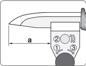
The edge angle on the tip is depending on where the jig is mounted on the blade (a). If it is mounted towards the handle, the edge angle at the tip will be smaller. If the jig is mounted towards the tip, the edge angle at the tip will be larger.
