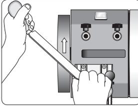
*Hone free-hand. Hold the knife diagonally to clear the grinding wheel. Hone the bevel and the reverse side alternately.*
