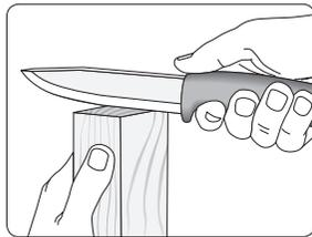
You can ensure that the burr is completely removed by drawing the knife through a piece of end grain wood.
