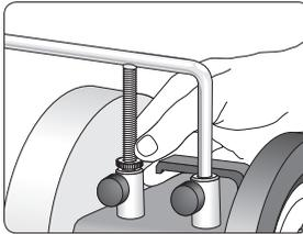
Raise the Universal Support with the Micro Adjust until the whole bevel touches the grinding wheel. Check by moving the wheel by hand to see where the grinding will take place.
