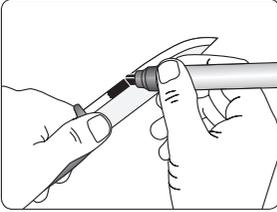
Colour the bevel with a marker so that you can see where the grinding will occur.
