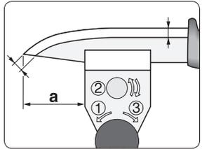
The correct mounting position (a) will make the bevel and the edge angle the same along the entire length of the blade.
