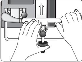
*Press the jig downwards so that the stop is all the time in contact with the Universal Support. Ensure that the grinding takes place across the entire width of the grinding wheel.*
