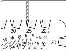
You can measure the edge angle in the grooves of the AngleMaster.
