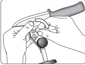
Adjust the jig with the small screw to fit the thickness of the knife.
