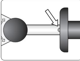
Turn the stop of the jig to zero.
