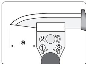
Short knives, which you can mount in the jig up to approx. 50 mm (2") from the tip (a), can be ground away from the edge.
