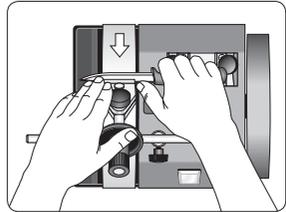
When the first side is ground, turn the jig upside-down – the knife is still fixed in the jig – and grind the other side. Now the burr appears immediately as it has already developed on the under side. Grind as much as on the first side to obtain a symmetrical edge.
